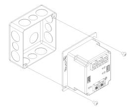
MOUNTS TO STANDARD 4"x4" ELECTRICAL JUNCTION BOX (JUNCTION BOX NOT INCLUDED)
